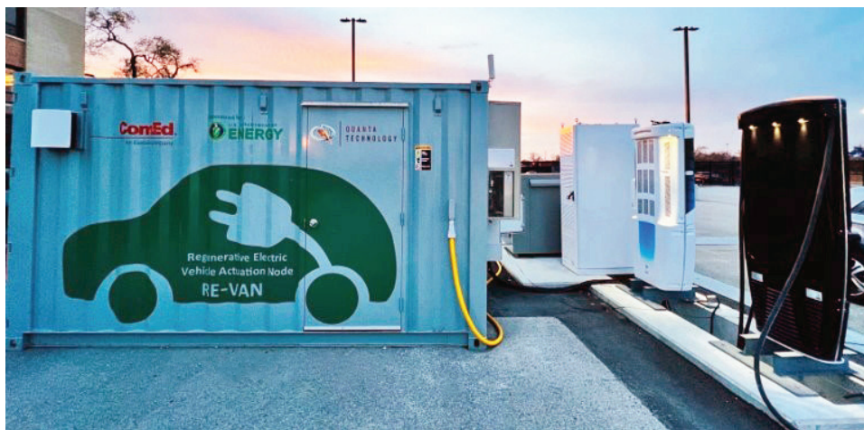
PICTURED: Outdoor lab setup for functionality testing DC fast and ultra fast charging stations using ultra-fast charger R-Series
