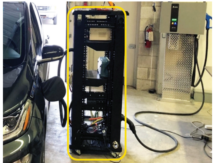
PICTURED: DC EV submetering lab testing using DC EVMT (laboratory version)
