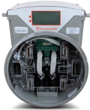
ConnectDER: behind-the-meter DER monitoring device
